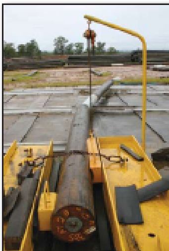
A range of KPOLE TSJ sizes were tested in the horizontal test rig at Koppers Grafton plant in February 2007
